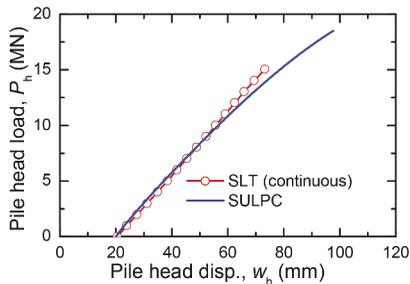
Figure 8. Static load-displacement curves from SULPC and SLT.
