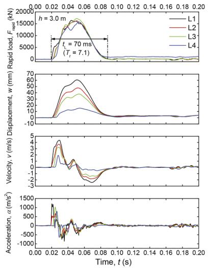
Figure 5. Measured dynamic signals ( $h = 3.0$  m).
