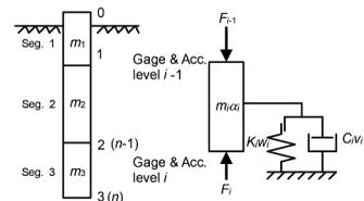
Figure 3. Segmental Unloading Point Connection (SULPC) method.
