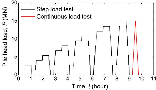
Fig. 5. Loading sequences in SLTs.
