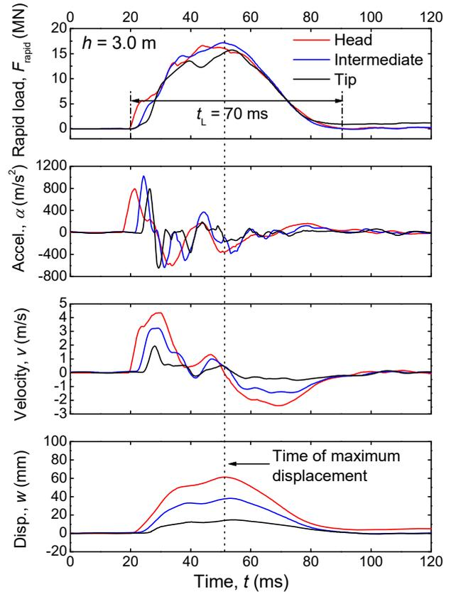
Fig. 7. Measured RLT signals in the last (7th) blow.
