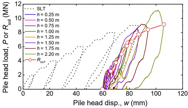
Fig. 14. Soil resistance vs. pile head displacement.
