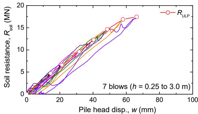
Fig. 8. Soil resistance vs. pile displacement in Type 2.
